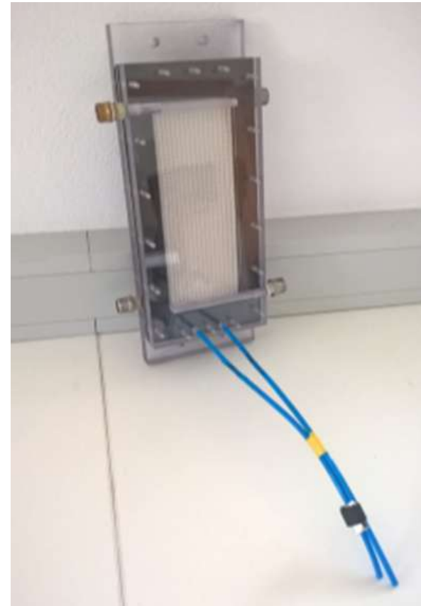
MD test module (effective membrane surface 25 \times 10 \text{ cm}^2 )
